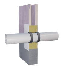
Flexi-Coat® is a highly advanced flexible penetration and aperture sealing system. The Flexi-Coat® is supplied in the form of both completed pre-coated Flexi-Coat® Fingers and as a coating to be applied to stone/mineral wool backing material. Flexi-Coat® has also been tested in accordance with EN1364-4 and is third party certified.
