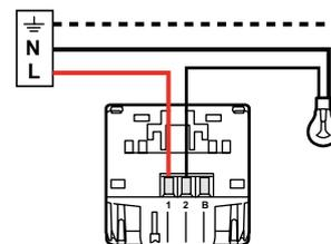
**5.2 Connection combined with one or several mechanical push-buttons**
