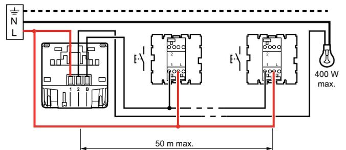
**Touch-control switch with no neutral 400 W****6. TECHNICAL DATA****6.1 Mechanical characteristics**
