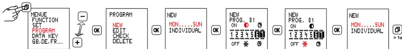
Within a specified switch-on/off time, the brightness determines the switching times
