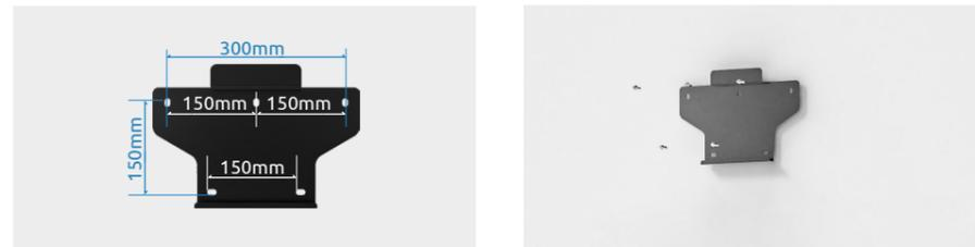
Insert the expansion tubes into the holes and tighten them, then fix the bracket onto the wall with expansion screws by using a cross screwdriver. Lift up the inverter with both hands, hang the back rail on the fixed wall bracket carefully.
