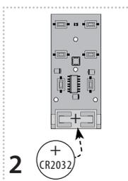
Slide the CR2032 battery into the battery holder. Observe the polarity.
