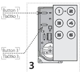
Insert the device into the bottom cover. Attach the front of the cover and click.
