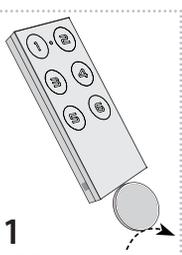
Use a coin to open the key fob and remove the front cover. Carefully tap the device out of the bottom cover.
