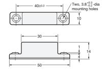
Note: The shape of the magnet is the same for Pre-wired Models and Terminal Block Models, but the magnet specifications are different.
