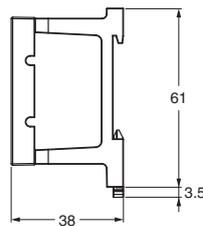
This Adapter is used to mount the E5CD to a DIN Track. If you use the Adapter, there is no need for a plate to mount in the panel or to drill mounting holes in the panel.
