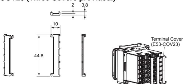
The Terminal Covers are provided with the Digital Temperature Controller.
