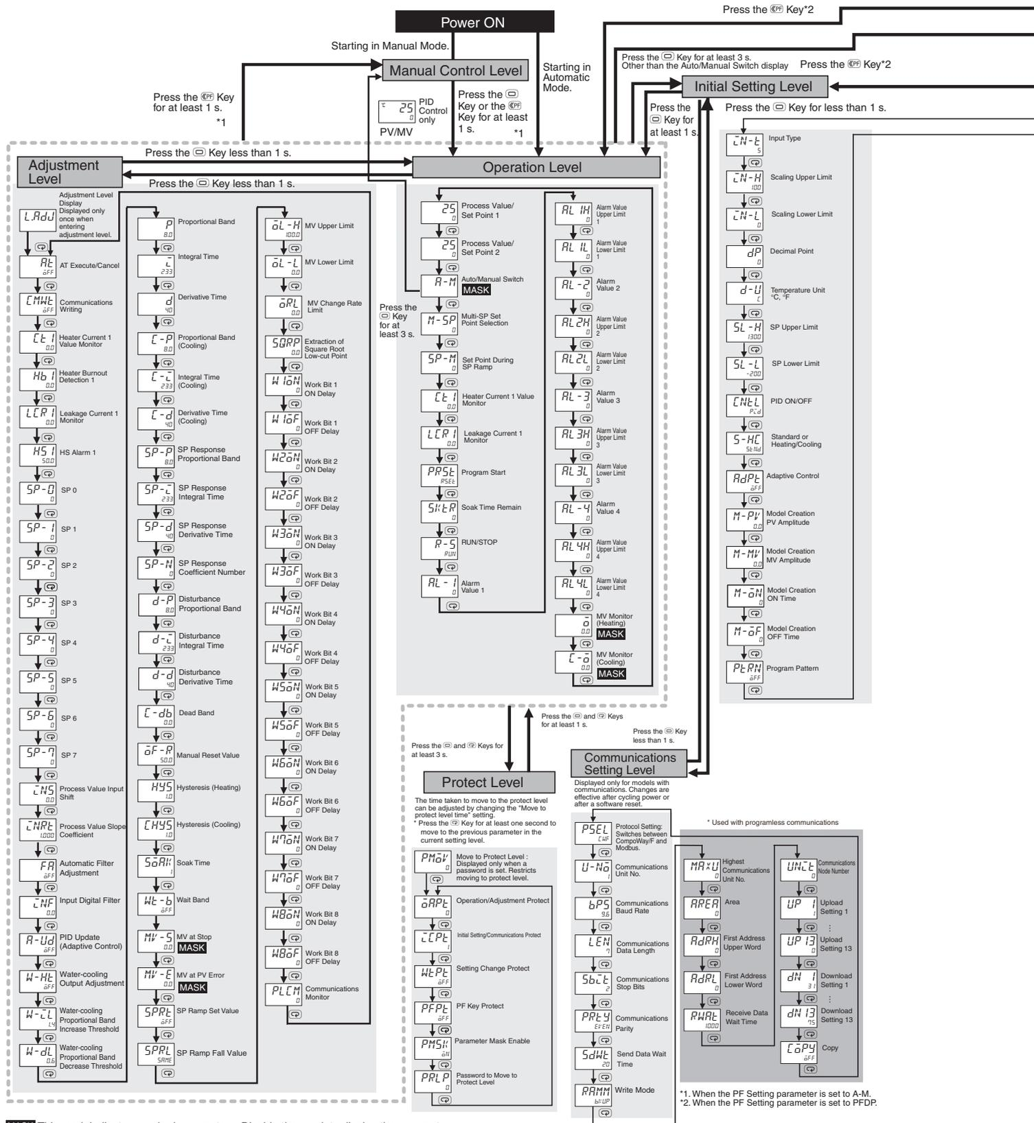
**MASK** This mark indicates masked parameters. Disable the mask to display the parameter. Refer to 5-12 Hiding Parameters in the E5□D Digital Temperature Controller User's Manual (Cat. No. H224).
