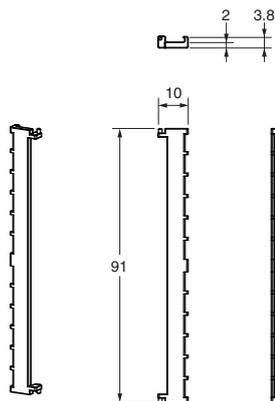
The Terminal Covers are provided with the Digital Temperature Controller. Order the Terminal Cover separately if it becomes lost or damaged.
